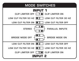
Fig. 3.4: DIP switch positions for parallel operation
