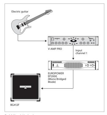
Fig. 3.5: Mono-bridged mode
