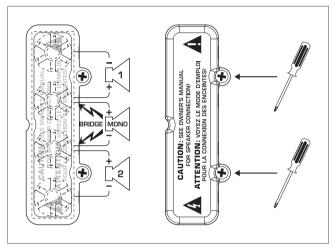
Fig. 4.2: Protective plastic covers shielding the binding posts
