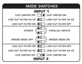
Fig. 3.2: DIP switch positions for 2-channel operation
