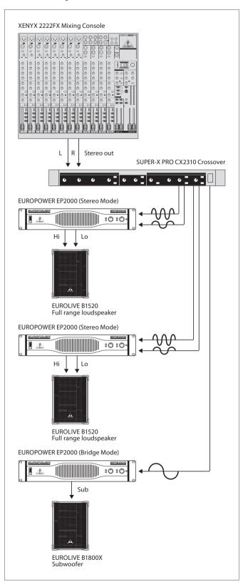
Fig. 3.7: Stereo bi-amp mode with a separate subwoofer
