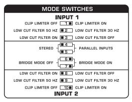
Fig. 3.6: DIP switch positions for mono-bridged mode
