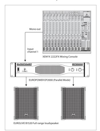
Fig. 3.3: Parallel operation
