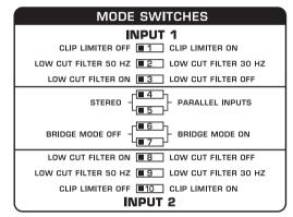
Fig. 2.3: Dip-switches
